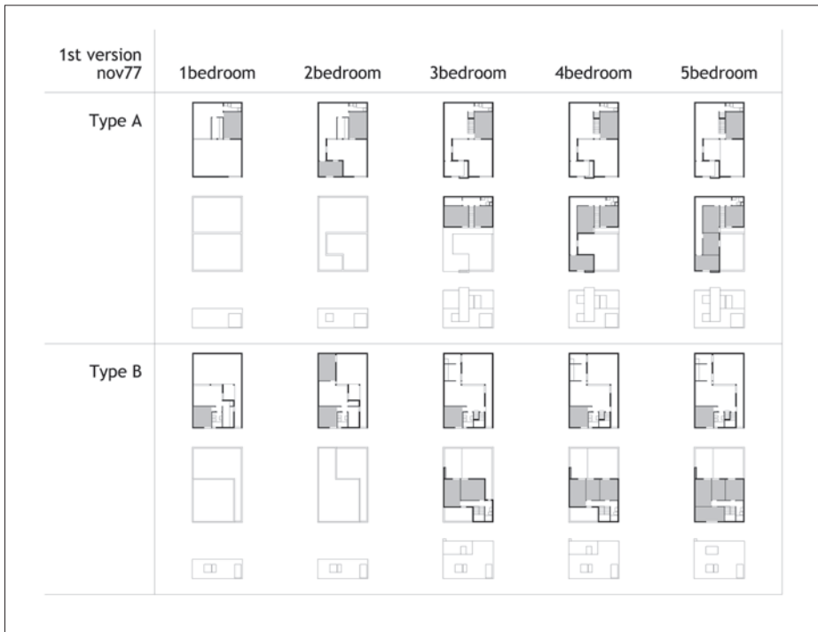
First version of the dwelling types for the Malagueira Neighbourhood, November 1977. Source: Author's Drawing.
